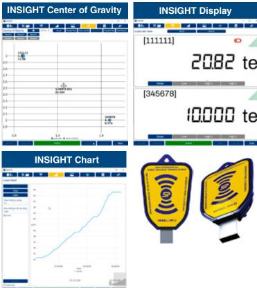
INSIGHT software, supplied with an SW-D USB wireless dongle, allows connection of up to 126 Crosby Straightpoint wireless loadcells simultaneously onto any Windows tablet or laptop.
