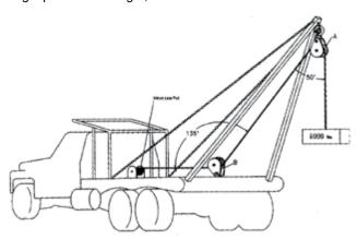
There is no mechanical advantage to a single part load line system, so winch line pull is equal to 1,000 lbs or the weight being lifted.
