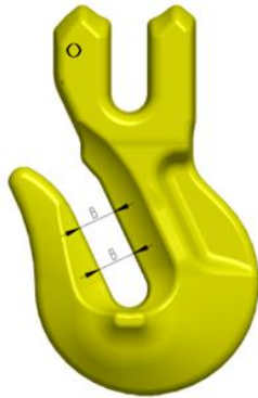
Figure 8: Chain slot is parallel
