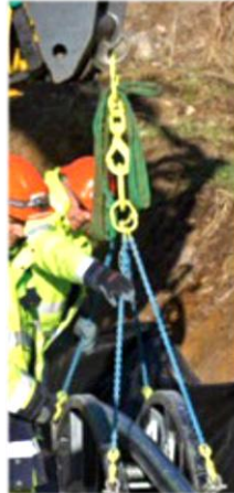
Figure 22: GrabiQ Chain lifting sling connected with swivel Hook BKLK, G-Coupling Link and top Master Link in crane hook
