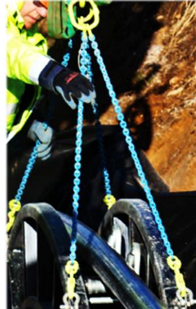
Figure 22: GrabiQ Chain lifting sling connected with swivel Hook BKLK, G-Coupling Link and top Master Link in crane hook
