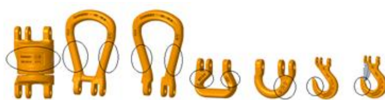
Figure 16: Recommended areas for punched or engraved marking
