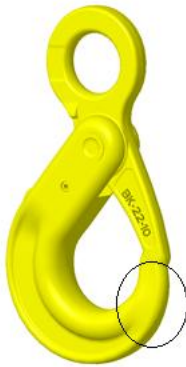
Figure 3: Recommended areas for punched or engraved marking
