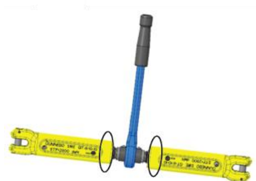
Figure 3: Recommended areas for punched or engraved marking
