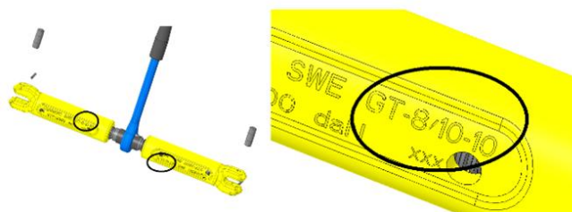
Figure 5: General marking on both GT-8-10 and GT-10-10
