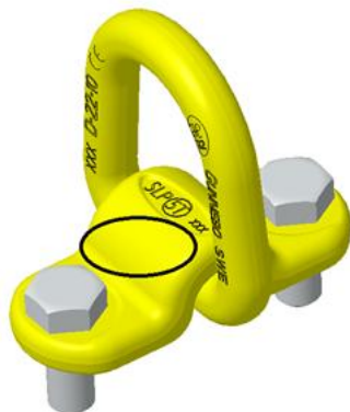
Figure 5: Recommended position for punched or engraved marking
